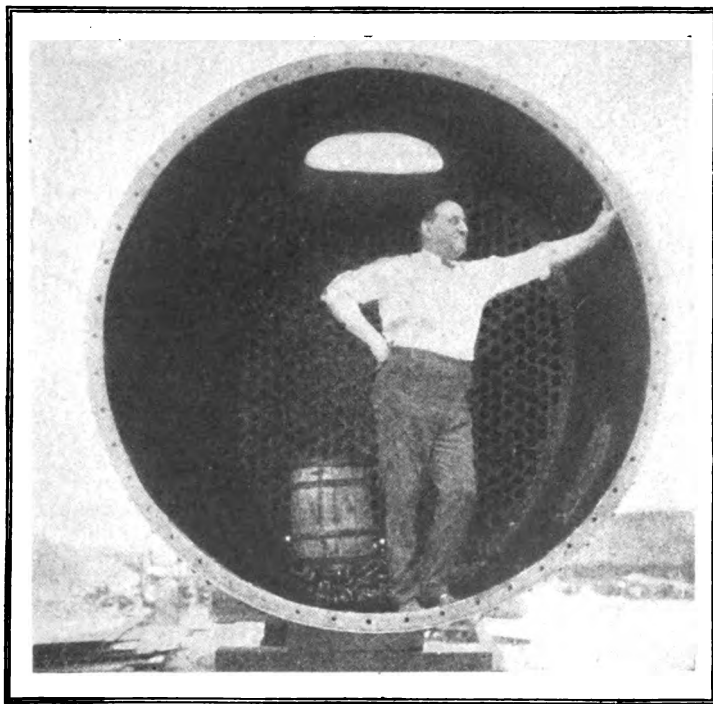
Mallet Articulated Compound Locomotive for the Erie—Smokebox
